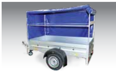
Tarpaulin and frame, load height 1000/1300/1600/1800 mm (size depending on model)
