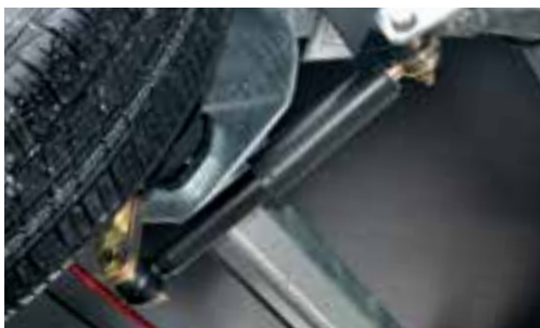
Wheel shock absorbers (mounted) incl. 100 km/h confirmation, wheel shock absorbers (loose) without 100 km / h confirmation
