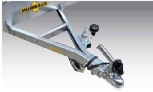
Crossbar (loose) for jockey wheel
